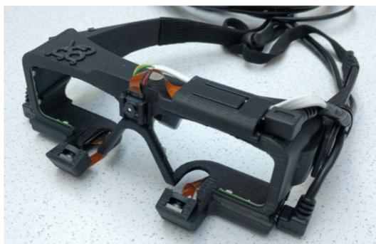
**Figure 2.** The gaze tracking glasses used in the study
